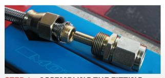
**STEP 4 - ASSEMBLING THE FITTING** Now it time to finish assembling the fitting. The first image below should give you an idea of what's next. But firstly we like to get a drop of lubricant on the fitting. Now you need to push the hose onto the fitting so the mandrel on the fitting goes inside the Teflon inner hose. Push the hose on all the way down so the olive meets the base.
