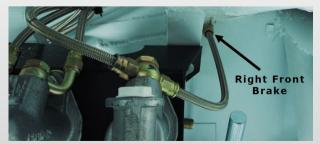
**STEP 5 – RIGHT HAND BRAKE CALLIPER** The brake hose for the right hand brake calliper. Again a bulkhead fitting is used.
