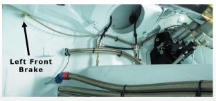
**STEP 4 – LEFT HAND BRAKE CALLIPER** The brake hose for the left hand brake calliper. Here a bulkhead fitting is used.
