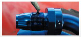
**STEP 4 - PREPARE THE FITTING** We have put some more masking tape on the exposed part of the hose. This is IMPORTANT, so we can see if the hose moves when we tighten it up at the next step. Next you should lubricate the thread on the fitting.
