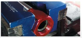
**STEP 3 – INSERT HOSE INTO FITTING** Remove the masking tape. Now we unscrew the hose end of our fitting. Then using a twisting motion push the hose into the back of the red part of the fitting. Once you've got it started off we recommend placing it in a vice. Keep pushing the hose into the fitting until the end of the hose is secured against the step inside the hose end.
