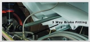
**STEP 6 – THE FINISHED HOSE** From the other side of the rear bulkhead fitting you can see the hose connects to the axle. (You must allow for movement of the axle, the car is sitting on sill stands in this picture) The 3 way brake fitting is fitted too the axle, splitting the brake line for left and right rear callipers. how to / setup rally brake hose
