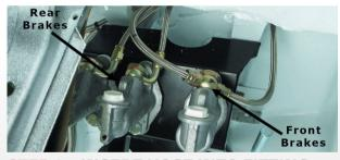
**STEP 3 – INSERT HOSE INTO FITTING** There are 3 master cylinders, 1 hydraulic clutch, 1 rear brake and 1 front brake. The fluid reservoirs are not yet fitted. The master cylinder on the right is for the front brakes. At win banjo is used to split the left and right front brake callipers. This is different to the diagram but acceptable. The middle master cylinder is for the rear brakes with a single banjo fitting.
