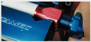
**STEP 5 - TIGHTENING THE FITTING** Then using your hands insert the fitting into the hose end and get it started on the threads. Once this starts to become tight use a AN spanner to tighten the fitting up.
