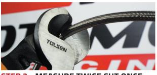
**STEP 2 - MEASURE TWICE CUT ONCE** Measure the amount of hose you want and then cut it. We have chosen to cut out hose using very sharp cutters. But if in doubt use a fine toothed saw, especially on thicker hose. As it's very important to have a very clean and straight cut.
