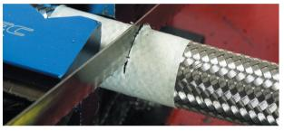
**STEP 2 - MEASURE TWICE CUT ONCE** As it's very important to have a very clean and straight cut, and with this thickness of hose, we recommend using a fine toothed saw and taping up the area to be cut with masking tape. This will reduce fraying on the stainless steel braid.
