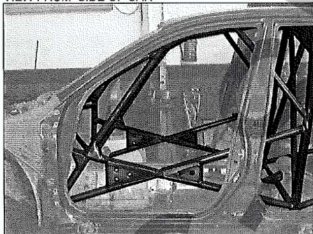
PHOTO 5 REAR BACKSTAY TO BODY ATTACHMENT
