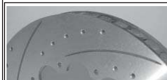
GD = Grooved & Drilled. Usually used on Road applications.
