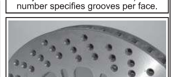
D & SD = Cross Drilled. (Drilled holes chamfered). Still preferred with some pad materials but can compromise disc life.
