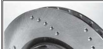
RD = Radiused Drilled. (Cross drilled but with radiused run out to reduce noise & improve life compared with standard cross drilling. Usually used on Road applications.
