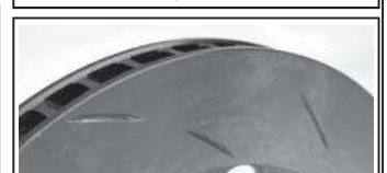
PG = Partial Groove. Shorter length groove pattern
