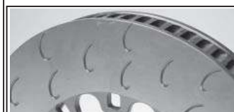
RC = 'J' Hook Design. As RA design but with 3 hooks across face. This design gives improved bite and debris clearance and reduces distortion / vibration. Thick wall discs only
