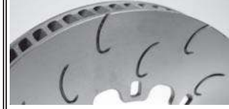
RA = 'J' Hook Design. Gives improved bite and debris clearance and reduces distortion / vibration, outer grooves run out to O/D. Thick wall discs only
